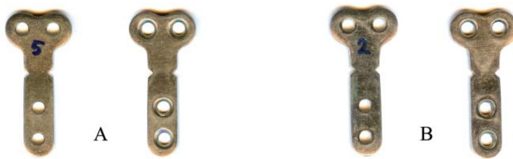
Figure 2 Both surfaces of the 316L stainless T plates fabricated for triple pelvic osteotomy; A: used plates, B: unused plates of the same production batch.
