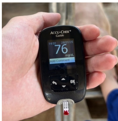
Figure 1 The portable glucometer used to measure blood glucose concentration in sows (Accu-Chek® Guide, Roche Diagnostics GmbH, Mannheim, Germany).
