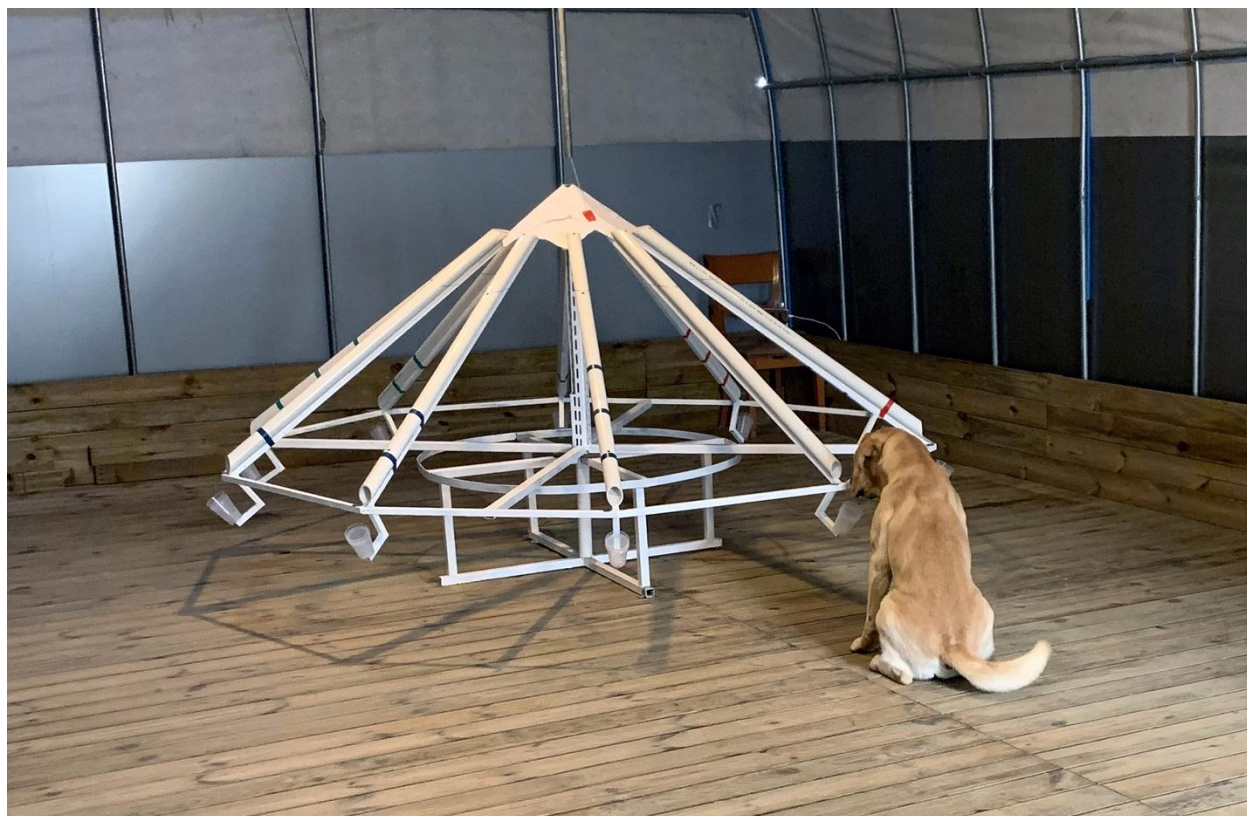
Figure 1 An experimental setup composed of a wheel with 10 ports and a scent-detection dog performing the training or test procedure.
