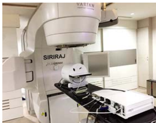
Figure 1. Machine set up. (A) aS1200 EPID and (B) PTW Octavius 1500 with 4D phantom.
