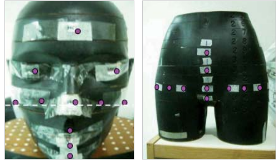
Fig 2. The measurements point of skin dose for head and pelvis area using TLD 100H
