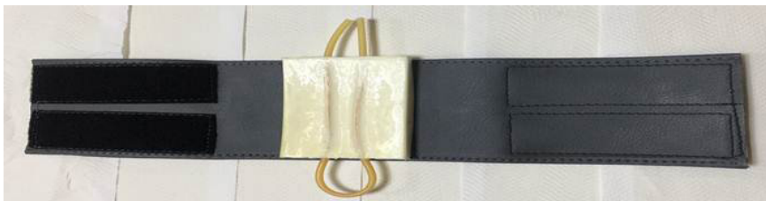
Figure 4 Attach the fake skin sheet to the rubber sheet using strong glue
