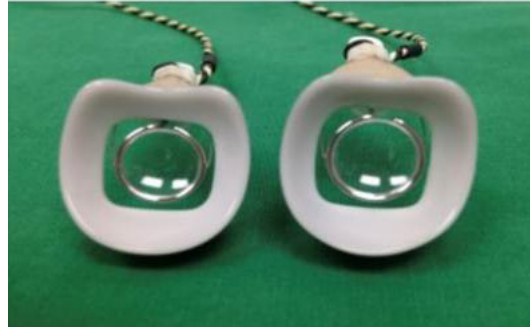
Figure 2 Contact lens electrode (CL electrode). Pediatric size (left) – for pediatric or small eye patient. Adult size (right) – for patient with normal size or large eye
