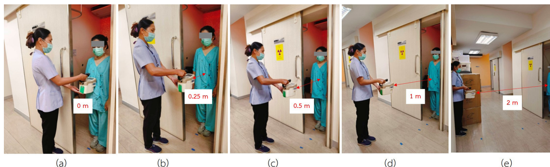
Figure 2 The measurer stands behind a lead door to measure the radiation dose rate from a patient undergoing an ^{18}\text{F} PET scan with a high energy of 511 keV (a) at a distance of 0 m, (b) at a distance of 0.25 m, (c) at a distance of 0.5 m, (d) at a distance of 1.0 m, and (e) at a distance of 2.0 m.
