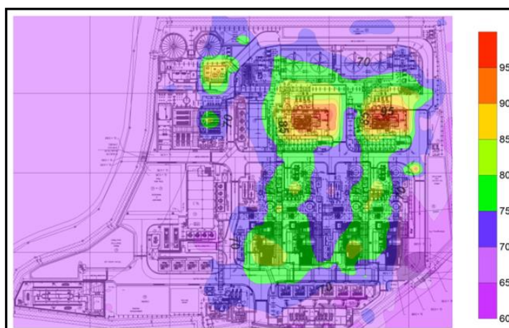
Figure 1 Noise Contour Mapping in power plant process
