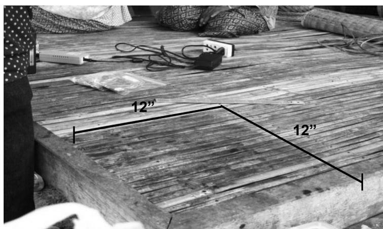
**Figure 3** Surface-wipe samples collection using Daniel's method [17]
