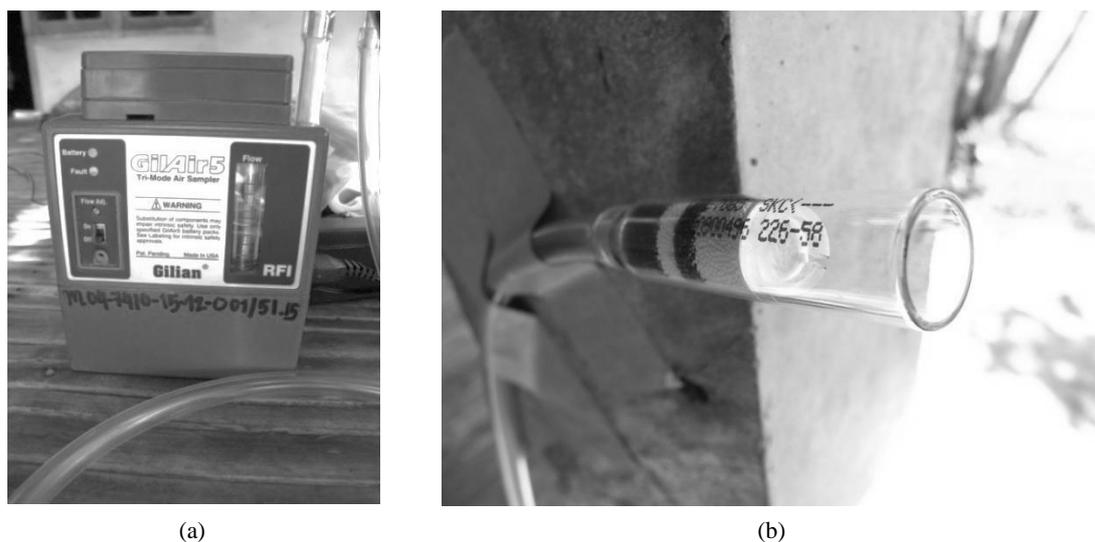
**Figure 2** Air Samples Collection by Using Personal Pump (a) and Collection Tube (b)
