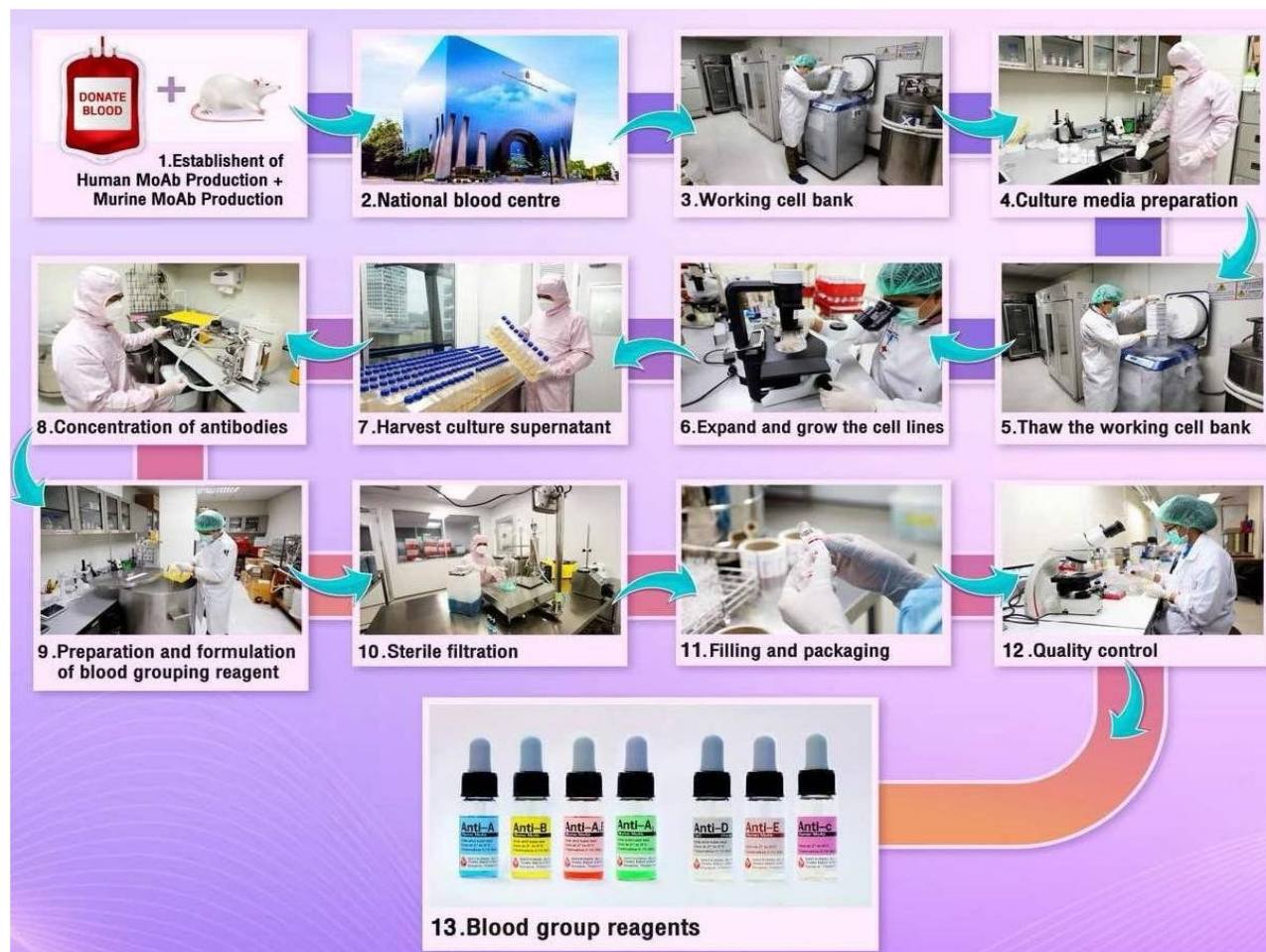
Figure 1. Summary of the production process of blood typing reagents by the National Blood Centre, Thai Red Cross Society.
