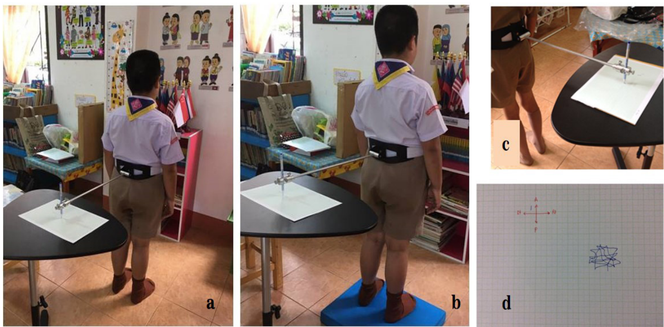
Figure 1 Assessment of postural sway using Swaymeter (a) on floor (b) on foam (c) Position of Swaymeter and pen on graph paper (d) Example of postural sway recording from Swaymeter.
