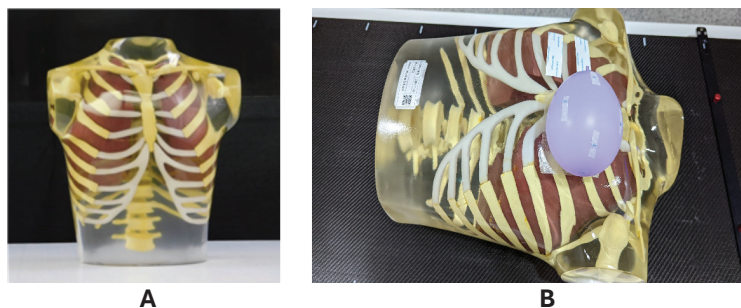
Figure 2. Breast phantom made using a thorax phantom and a water bag. A: thorax phantom, B: breast phantom.
