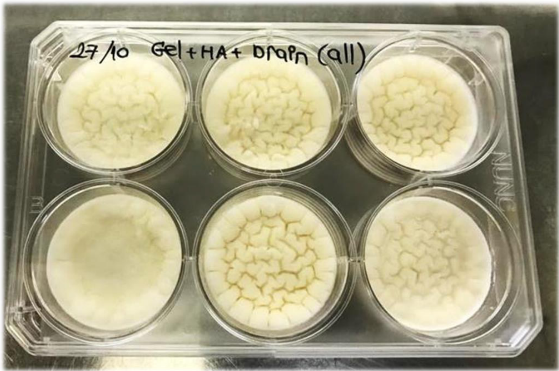
Figure 1. Lyophilized biomaterials made from 10% gelatin, 1 mg/mL nano-hydroxyapatite and pig brain extract (Gel + Ha + Brain).
