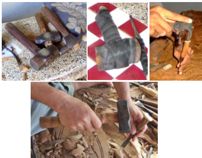
Figure 2. Conventional (Left) and modified tools (right). Hammer adapted for safe handling with grooves in the handle for fingers to fit and rubber wrapped around the hammer head and handle.
