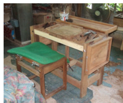
Figure 3. The innovative workstation with both table and stool for wood carving. Table is wooden and tilted with hand tool spaces in the front and on both sides. Stool was designed with an appropriate popliteal height and seat pan of appropriate width with a round ridge, and special adjustable tilt, in order to avoided contact stress.
