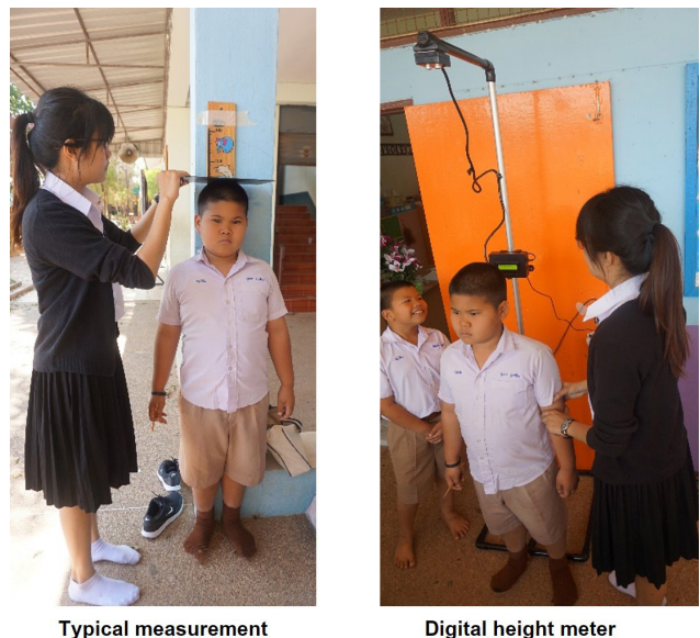
Figure 5 Measurement of height comparing between typical method and digital height meter.
