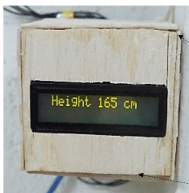
LCD to display the measured height
