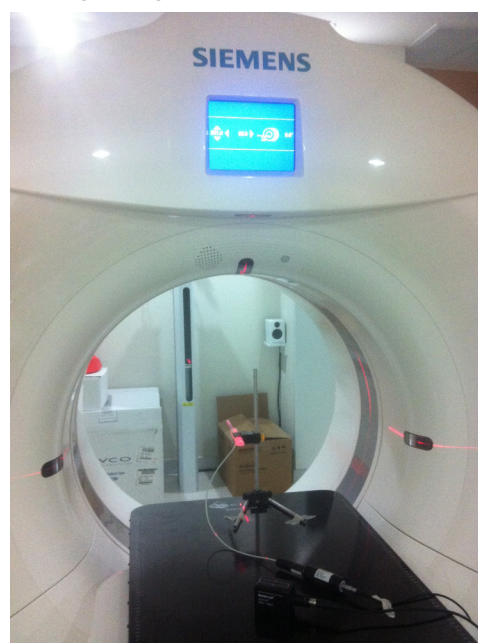
Figure 1 Setup of pencil ionization chamber for CTDI measurement in mid-air.
