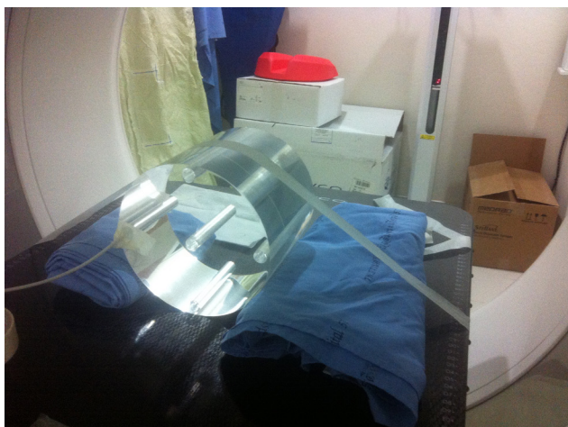
Figure 2 PMMA head phantom with 16 cm diameter was positioned for CTDI_{100} measurement in head protocol.
