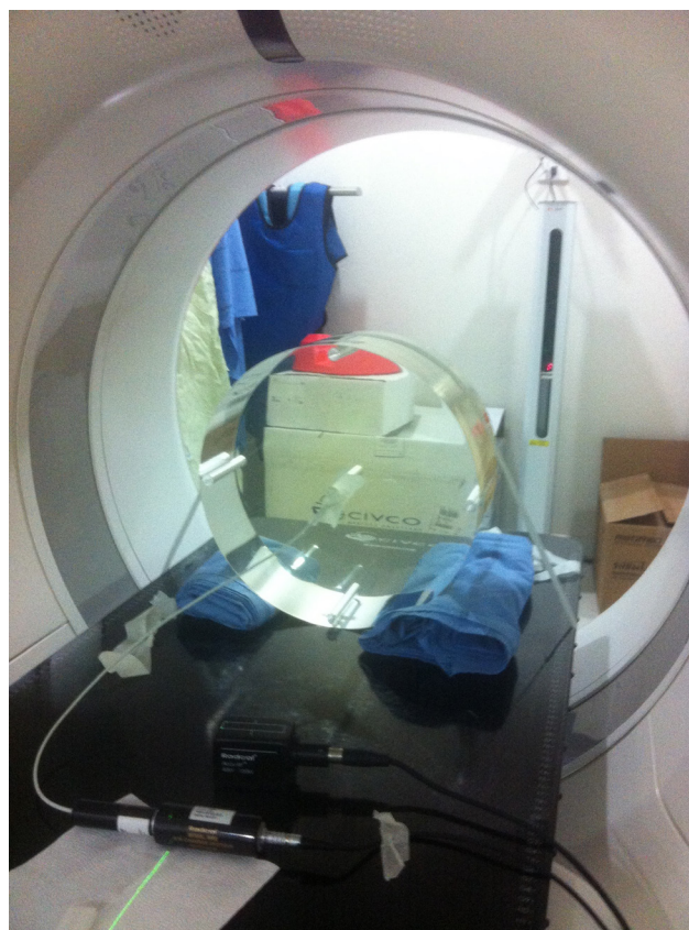
Figure 3 PMMA body phantom with 32 cm diameter was aligned with an isocenter for CTDI_{100} measurement in body protocol.
