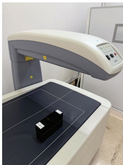
Figure 4. GE Lunar iDXA QC phantom used as the reference phantom for BMD validation.
