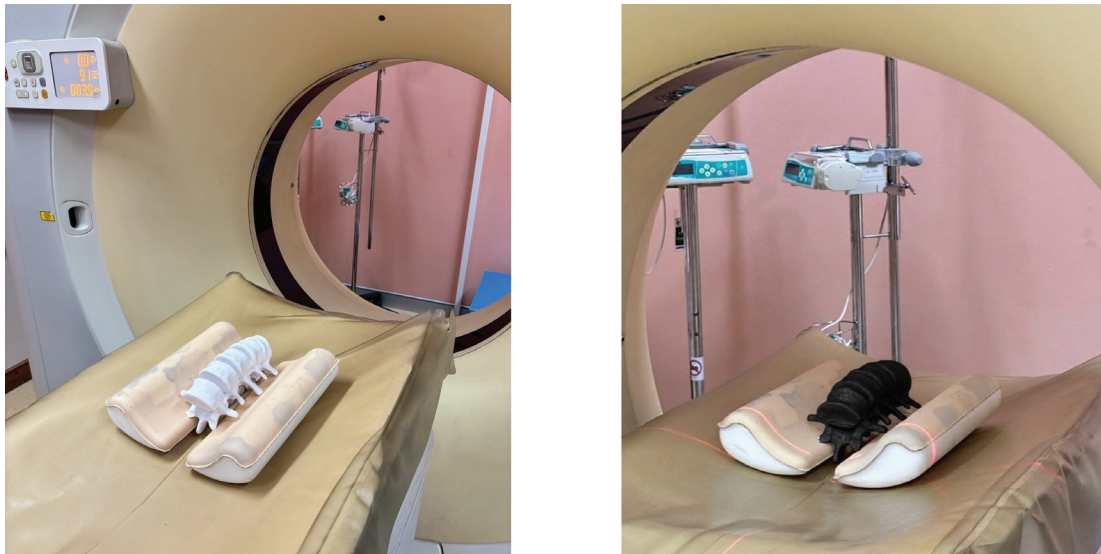
Figure 2. CT imaging of the developed 3D-printed lumbar spine phantom fabricated from PETG with calcium carbonate ( \text{CaCO}_3 ) powder with various material densities. Left: 1.24 \text{ gm/cm}^3 , Right: 1.27 \text{ gm/cm}^3 .
