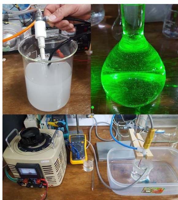
Figure 2. High-voltage stimulation in the micro/nano-bubble water system. (Figure was modified with copyright permitted from a previous publication 9 ).
