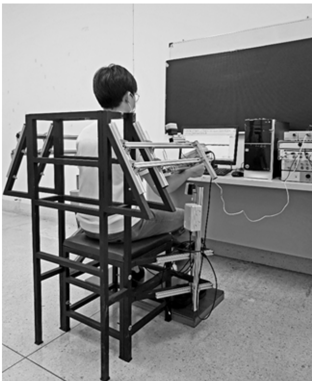
Figure 1. Participant position during maximal voluntary contraction (MVC) and force steadiness tests of 30 degrees of shoulder abduction.
