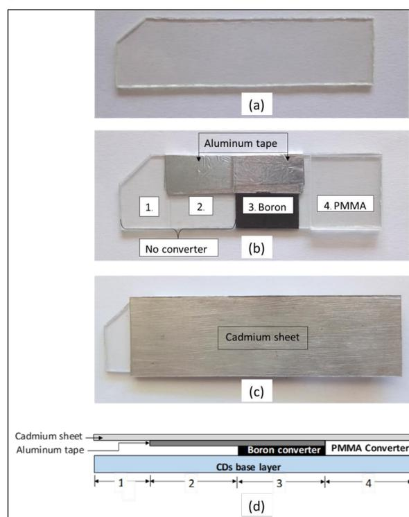
**Figure 1.** CDs track detector composed of first layer of a: CDs base (polycarbonate), b: second layer of various neutron converter, c: covered with cadmium sheet, and d: side view illustrating diagram of CDs track detector.
