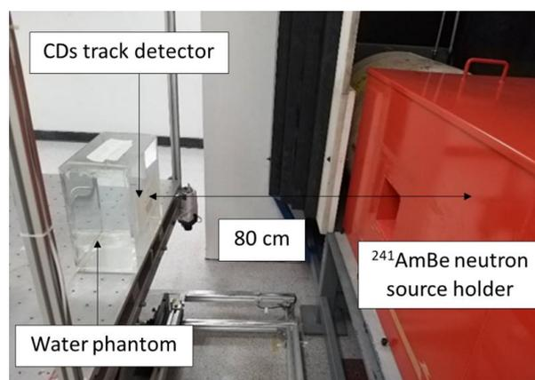
Figure 3. Fast neutron dose calibration set up.
