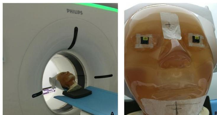
**Figure 2.** A head phantom on the head support (A) and the locations of OSLDs for the measurement of ESAK to eye lens (B).
