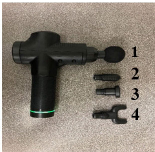
Figure 1 The handheld percussive massage gun with the different attachment heads: (1) hard ball head, (2) spinal head, (3) hard plain head, and (4) double-spinal head.
