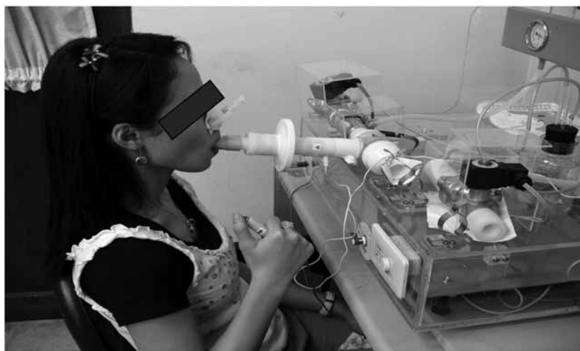
Figure 2 Respiratory resistance training device. Subject presses control button to start the experiment.
