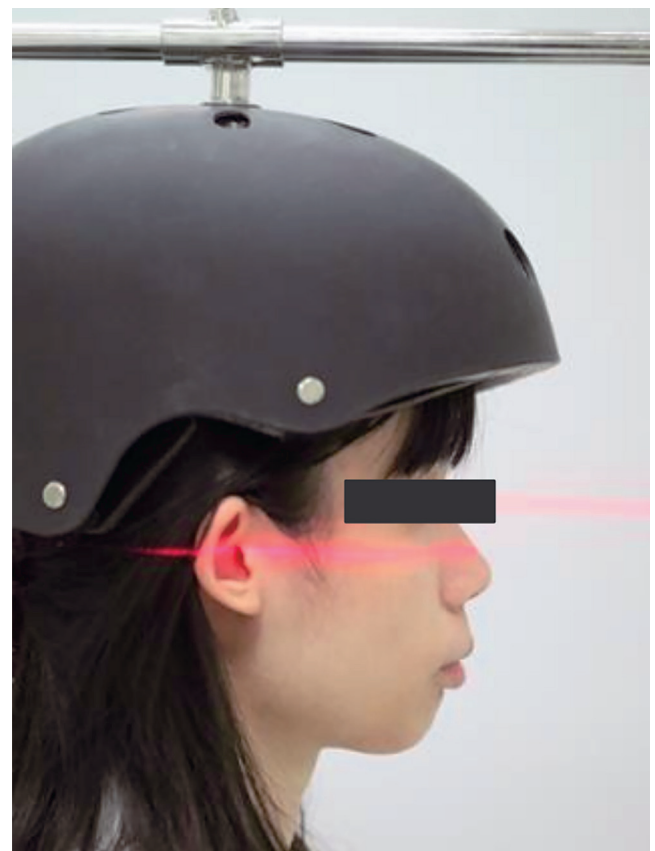
Figure 2 The head fixer and laser pointer referenced at the Frankfort horizontal plane
