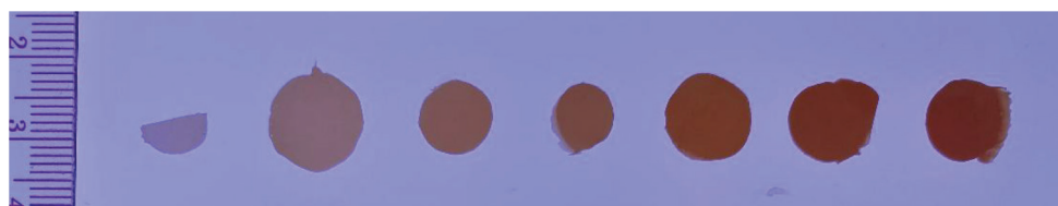
Figure 2 PVS material in known thickness placed together on a lightbox (50, 100, 150, 200, 250, 300, 350 \mu\text{m} )
