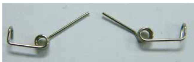
Fig. 1 The uprighting springs. A. Clockwise rotation B. Counterclockwise rotation
