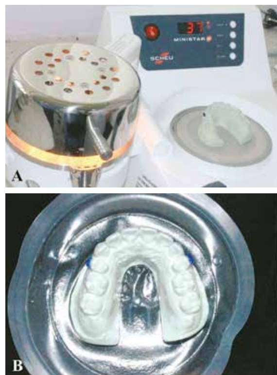
Figure 2. A. The vacuum thermoforming machine and B. the forming clear retainer.
