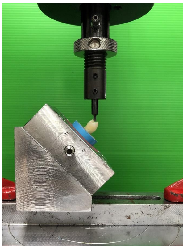
Figure 2 Simulated occlusal loading using a 2-mm-diameter handpiece along the axio-occlusal line at a 45° angle to the long axis.
