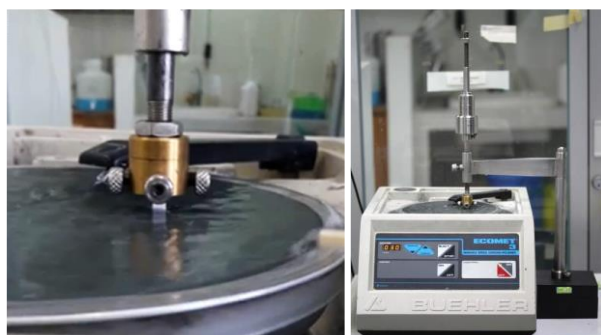
Figure 4 Specimen holder with polishing machine that used for wear resistance test.
