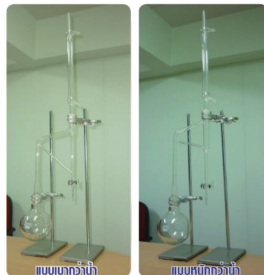
Figure 4 Clevenger apparatus for hydrodistillation
