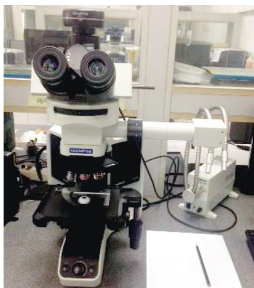
Figure 3 Trinocular microscope with camera and drawing tube
