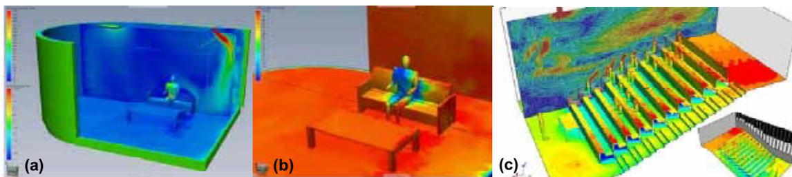
**Figure 5** Example of PMV value and velocity slice plane (a) and PPD result (b) of thermal comfort simulation result: (Autodesk Simulation CFD 2013) and Example of surface irradiation (c) of main lecture room: (STAR-CCM+ Building services 2013)
