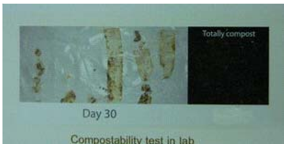
Figure 2 Biodegradation process of EcoAbsolute film strip until the completion of composting process
