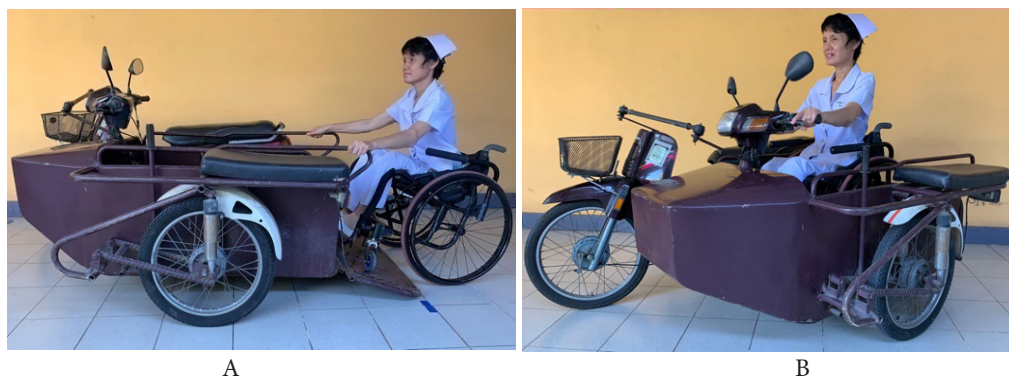
Figure 1. The modified motorcycle with a sidecar for wheelchair users designed by the Department of Rehabilitation Medicine, Faculty of Medicine, Chiang Mai University in 2004. (A) The wheelchair user rolls up the ramp by holding the side rails and pulling themselves along. (B) The wheelchair-seated rider controls the motorcycle with handlebars installed at the front of the sidecar.
