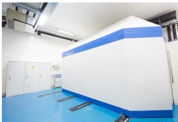
Figure 2. HM-20S vertical plane, self-shielded cyclotron (Sumitomo Heavy Industries, Shinagawa City, Tokyo, Japan) in the negative-pressured cyclotron room
